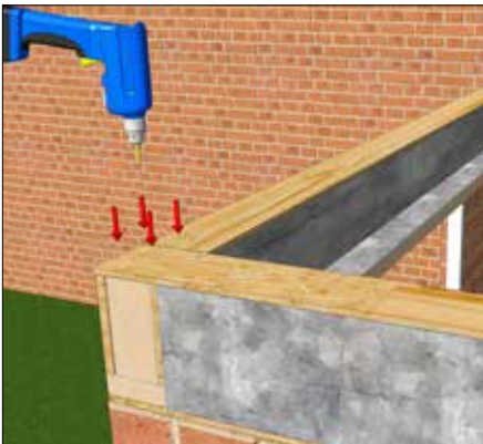
4x fixings GPHS050 required to screw through the top of the OSB into each external corner.
