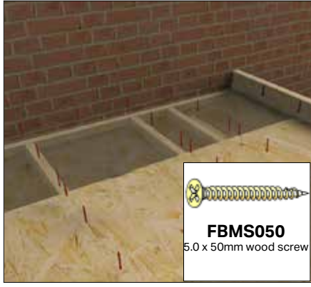
Use the screws provided to secure the board down into the firrings at 300mm centres.
