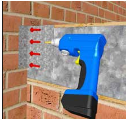
Push the loosely fitted abutment brackets up to host wall. Fix into the solid masonry with 4 suitable fixings (NOT SUPPLIED) avoiding mortar joints on both sides.
