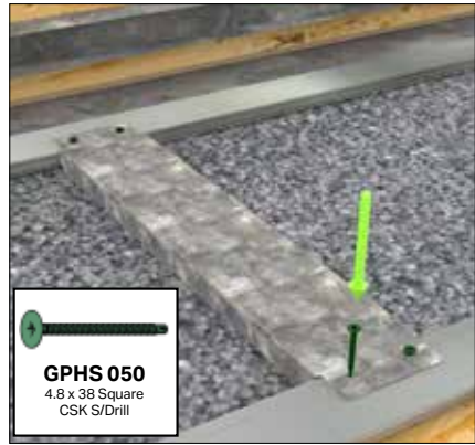
Pitchlock supports are shown in the Pitchlock location plan. They're fixed down with 4x GPHS050 screws into the predrilled holes.
