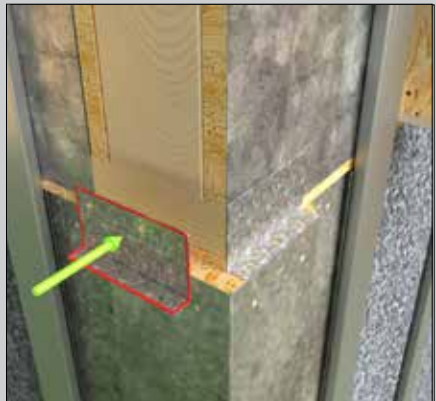
Detail specific to hup! jobs. Take 2 corner fixing brackets for each corner. Push them up against the front face of the beam and sit them on the corner post.
